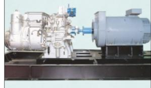
51H mounted on Kawasaki gas turbine engine.
