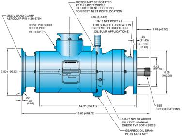
The Model 56K-LP is lightest and most powerful in its class. It is also designed to replace aero-derived starters costing thousands more. Excellent availability, powerful performance, and a high tolerance for contaminated air supplies creates a solid value for application on GE gas turbine engines.
