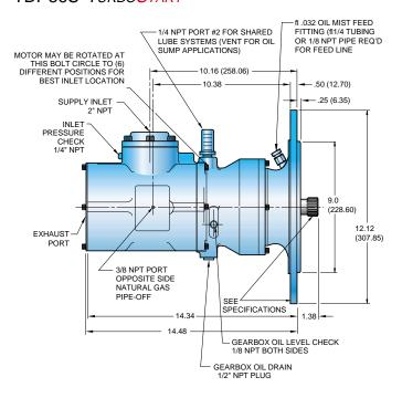
Our Model 56S is designed to mount directly to Solar Saturn engines. An integral soft clutch eliminates the jaw-type clutch assembly, for trouble free operation. And because the 56S motor requires no lubrication in the drive air...fugitive starter exhaust emissions can be totally eliminated.
