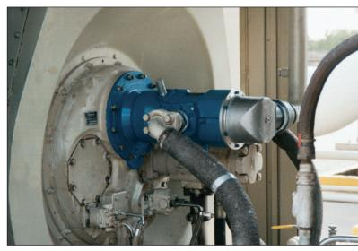
56S mounted on Solar Saturn engine.
