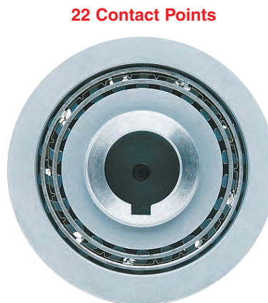
TDI's sprag clutch uses 22 evenly dispersed contact points that allow full crank starting and promote smooth engagement without the need for temperamental ramping controls.
