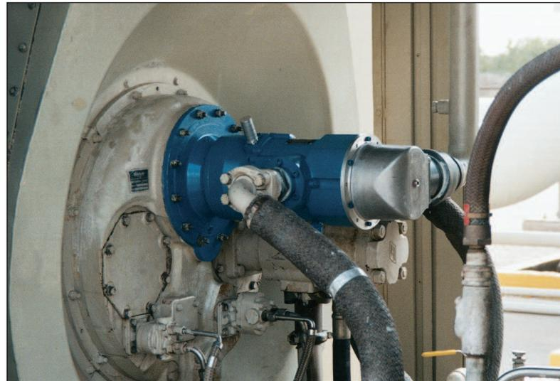
56S mounted on Solar Saturn engine.
