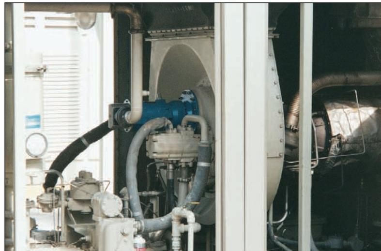
56S mounted on a Solar Saturn engine.
